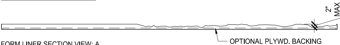
FORM LINER SECTION VIEW: A
