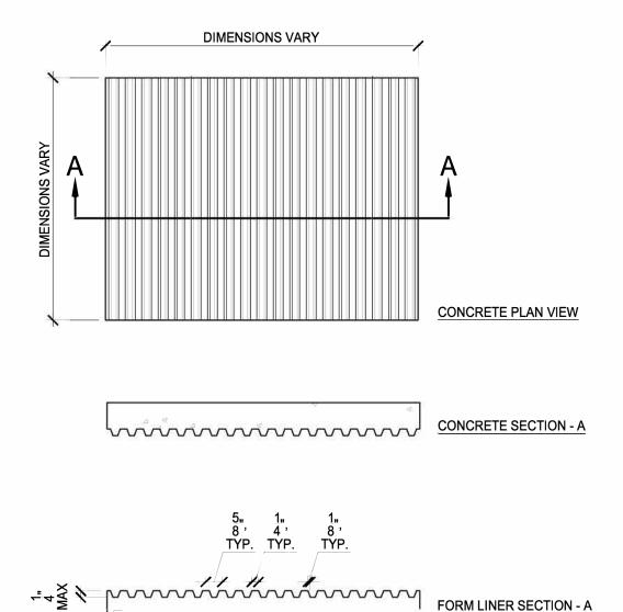
NOTE: FORM LINER THICKNESS VARIES ACCORDING TO THE SIZE OF THE PANEL.
