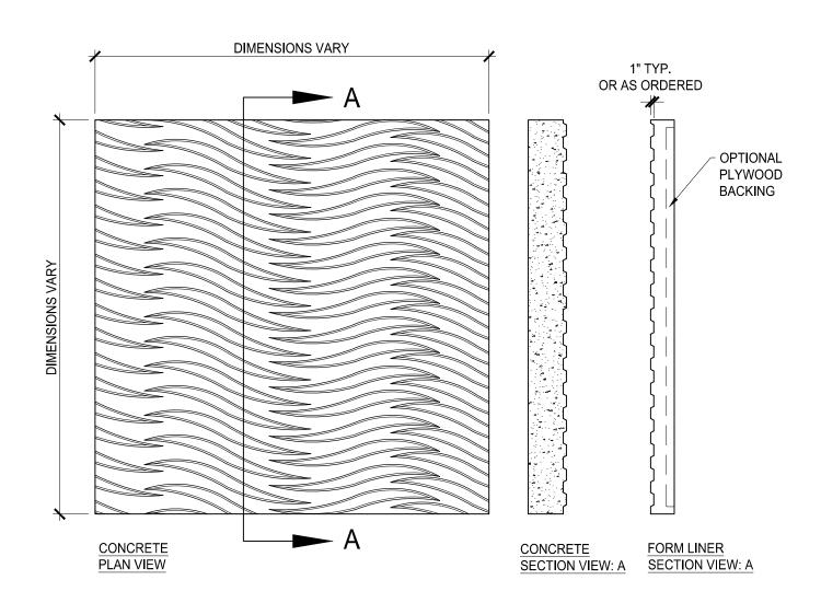
NOTE: FORM LINER THICKNESS VARIES ACCORDING TO THE SIZE OF THE PANEL.
