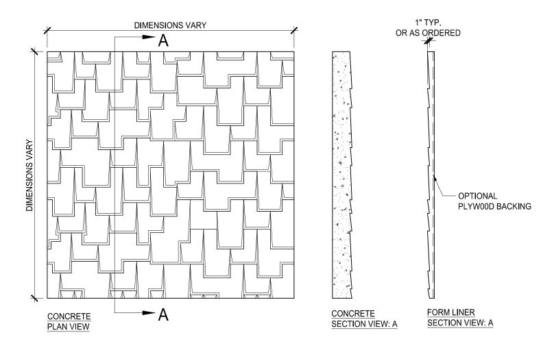
NOTE: FORM LINER THICKNESS VARIES ACCORDING TO THE SIZE OF THE PANEL.
